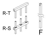
R-T:One-side-holes rail R-S:Through- holes rail
