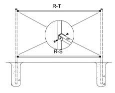
3. Install the rails into the brackets with screws.
